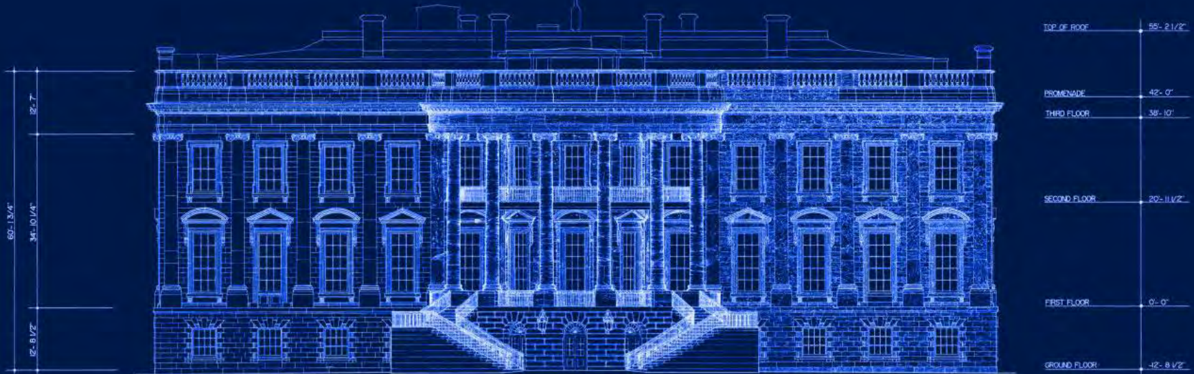
FULL ELEVATION ELEVATION SHOWING GRAIN PATTERN OF AQUA SANDSTONE NOTE: STONES WITHOUT GRAIN PATTERN WERE PAINTED OR INACCESSIBLE AT TIME OF RECORDING
